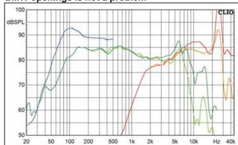
The Musway components run balanced and without interference in the important frequency range. The metal tweeter peaks at a high 25 kHz. The woofer pleases with a lot of sound pressure
