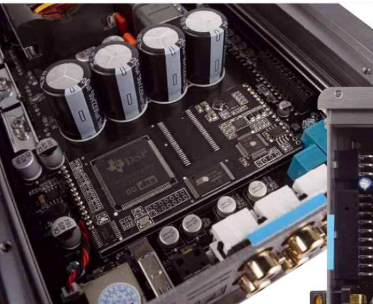
The M4+ is very clearly structured. The DSP components are on an extra circuit board
