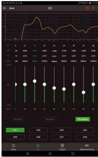
The app offers almost full functionality, here with equalizers and frequency response display
