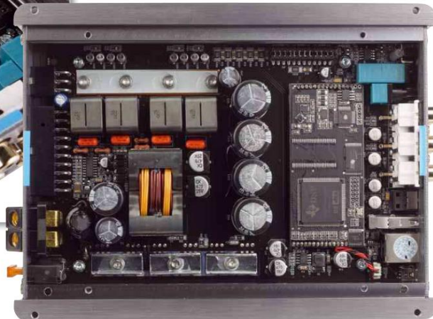
The M4+ is very clearly structured. The DSP components are on an extra circuit board
