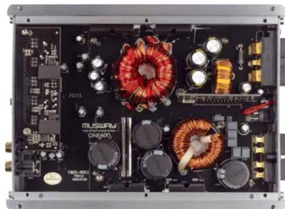
Nicely made heatsink with rounded edges, tidy inside and with Thick wire coils
