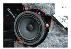
After removing the door panel, the speaker is freely accessible and can now be removed.
