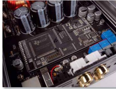
The 6 channels are amplified with 3 chips. The DSP sits with controller and memory on an additional board
