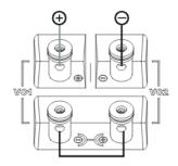
Connect amplifier at VC1 + and VC2 -140 - 220 Watt RMS, 4 Ohms Connect VC1 - with VC2 +
